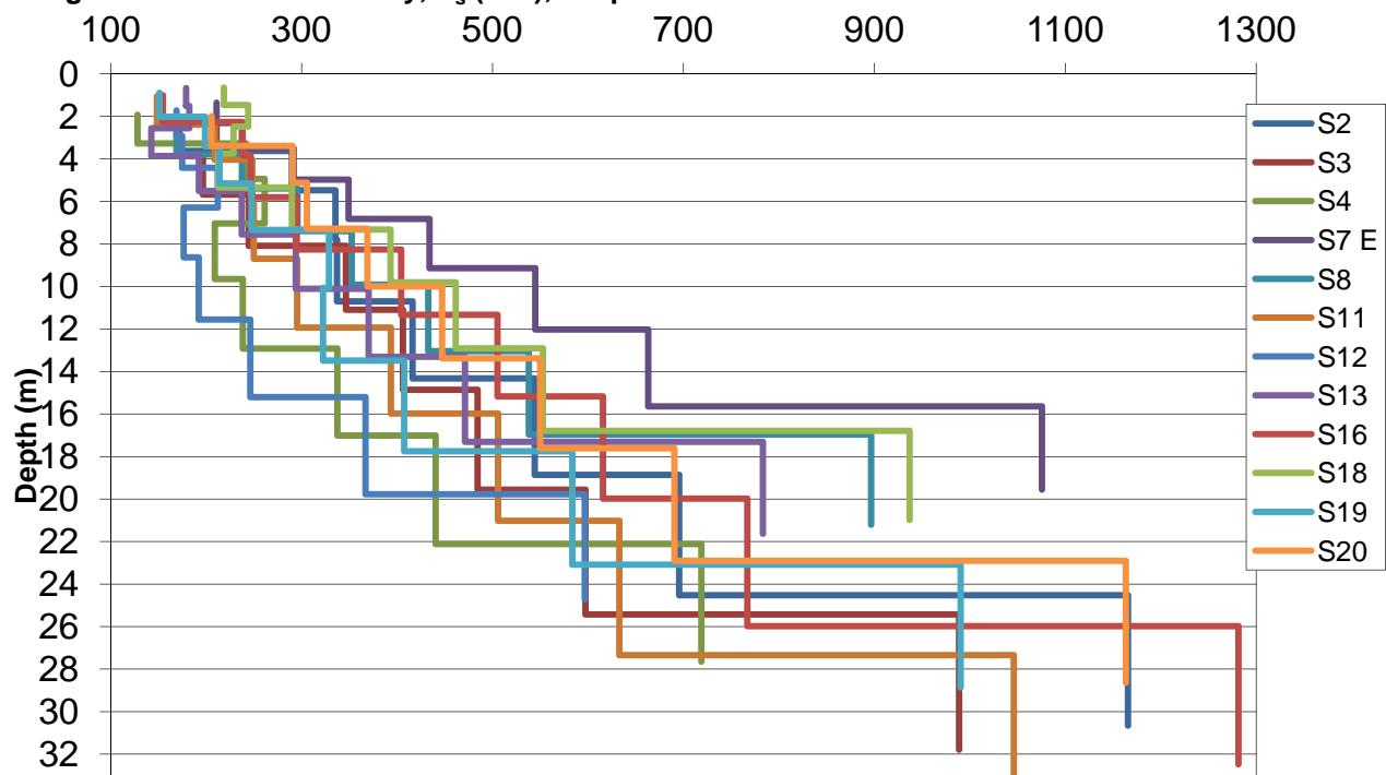
**Fig.3.3 Gmax, MPa, shallow bedrock**
