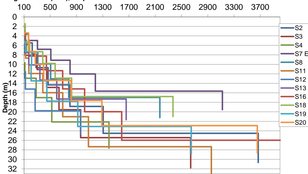
The 1D MASW Profiles show the variation in shear wave velocity with depth, at the centre of the profile location.
