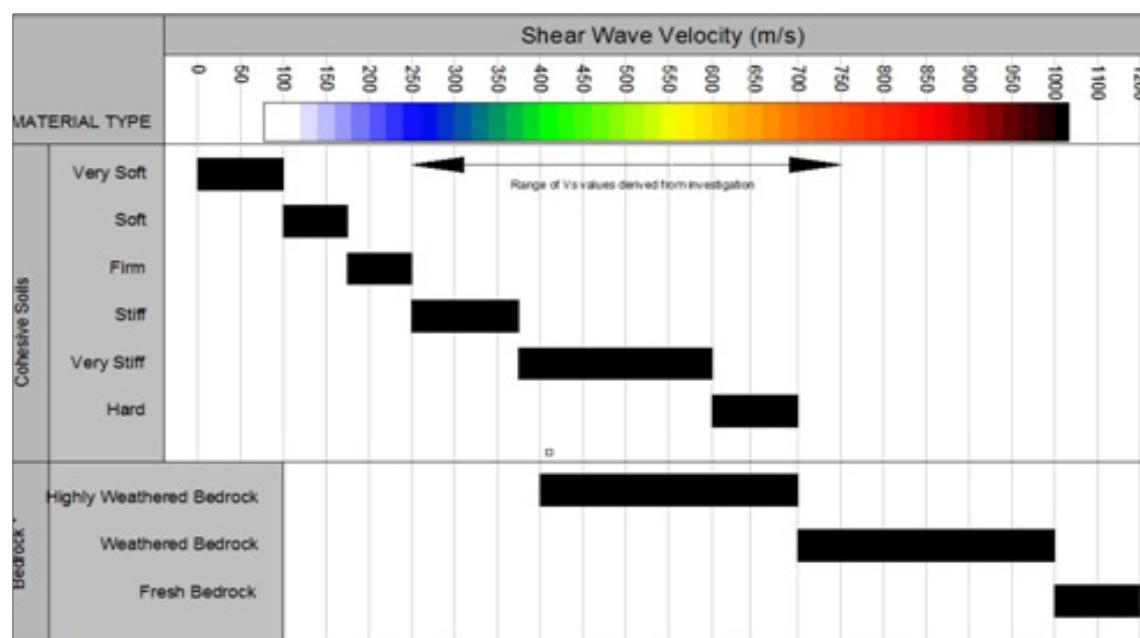
Fig.3.5 Shear wave velocity and corresponding soil stiffness.
